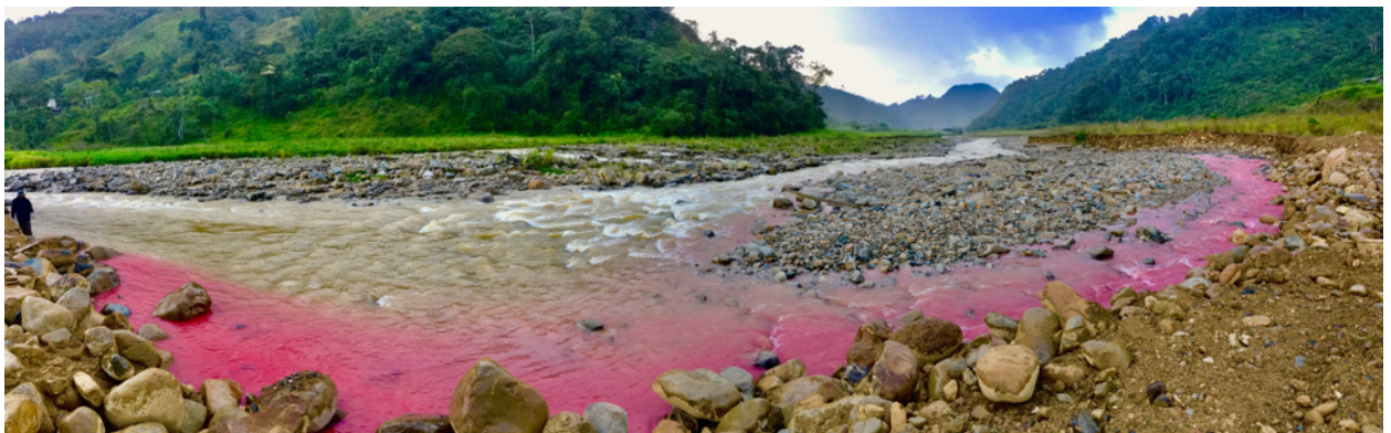
Conducting a tracer test on the Rio Nambija (Photo credit Sam Lopez)
