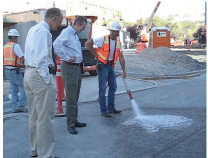
Onlookers watch in amazement as water from a full-blast fire hose is absorbed by pervious cement.
