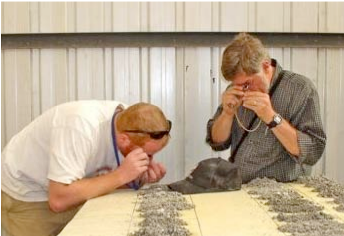
John Porter and Dr. Erich Petersen examine rotary drill cuttings from the El Peñon hydrothermal system.
